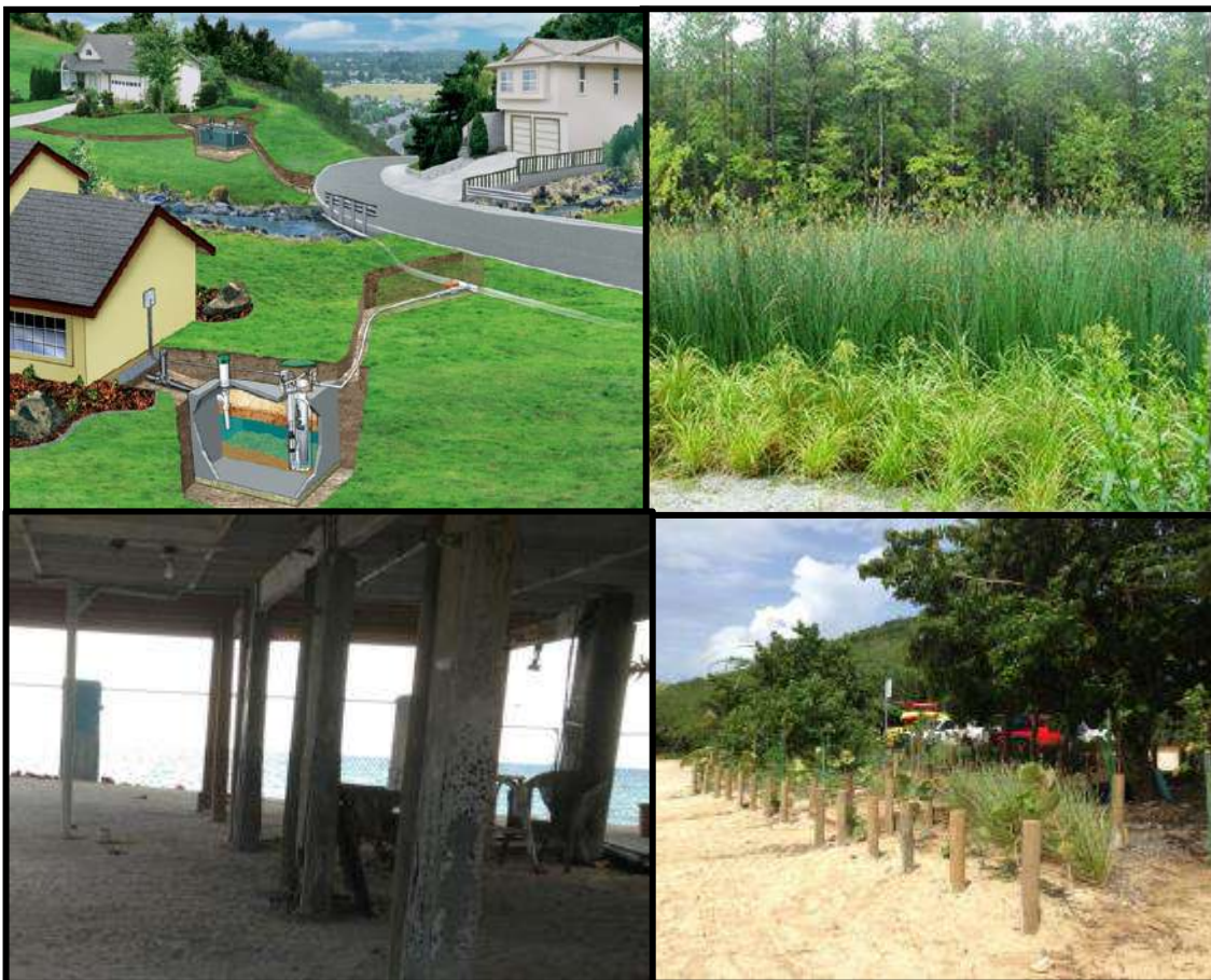
Figure 14. Top (Pump and treat system where effluent is pumped from homes to a constructed wetland or landscaped area (right); Bottom: (left) sewage effluent enters a septic system in the beach berm in Combate, (Bottom left) a passive low cost approach to addressing this issue is to restore a vegetated beach berm to include the use of vetiver and native species such as sea grape (uva playa) as has been done in Tamarindo Beach in Culebra
