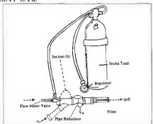
The pressure of the fluid coming through the reductor must be greater than the sum of the pressure drop of filters in use, however, since the filter will tend to clog at a time x due to the viscosity of the fluid, experimental work would always be needed to define the filtering capacity (The capacity of retaining a certain weight of particles from a specific volume of fluid) of different filtering materials. Samples can be recovered backwashing the filters.
