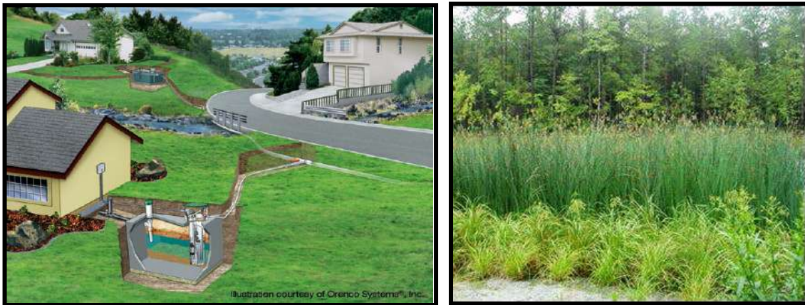
Figure 19. Pump and treat system effluent is pumped from homes to a constructed wetland or landscaped area
