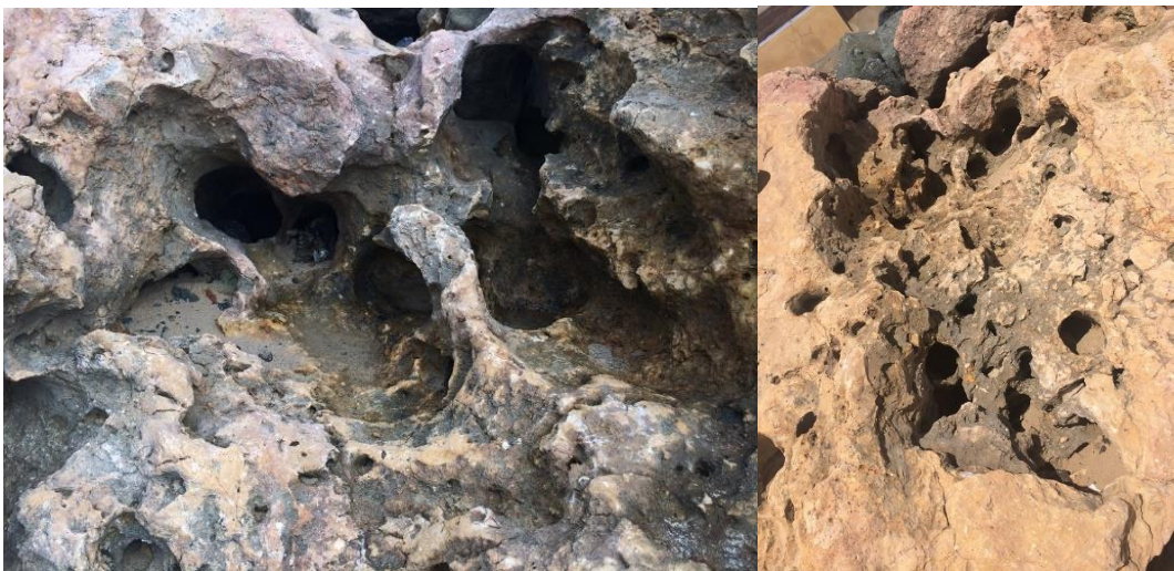
Figure 17. Naturally occurring crevices and pockets in aggregate suitable for artificial reefs and submerged breakwaters.
